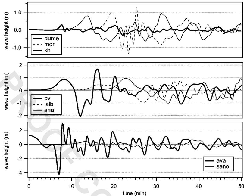
**Figure 6.** Wave gauge records for the full seven-segment Catalina Fault ( $M_w=7.6$ ) earthquake (Case 1). Note that the Avalon record starts above zero because the gauge is in the zone of tectonic uplift.
