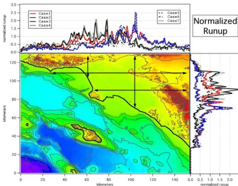
**Figure 10.** Map showing maximum runup normalized to the maximum seafloor/island uplift for each of the seven Catalina Fault tsunamigenic earthquake scenarios modeled in this study (fault parameters in Table 4).
