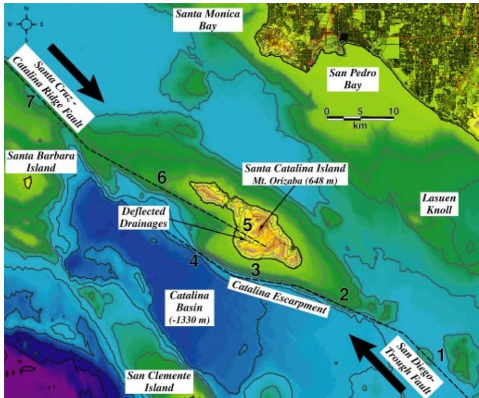
**Figure 3.** Contour map of the Santa Catalina Island “pop-up” structure. Seven segment Catalina Fault used for the tsunami earthquake models is shown. Large arrows show relative dextral motion across the Catalina Fault that creates transpression at the restraining bend. Deflected drainages suggest existence of right-slip fault aligned with the Santa Cruz–Catalina Ridge that cuts through the island.
