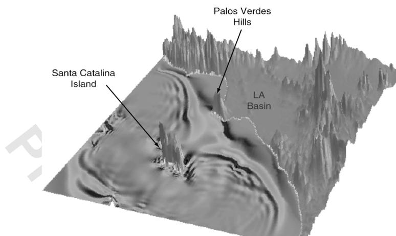
**Figure 7.** Time step in the MOST tsunami propagation simulation showing the two principal wave fronts generated from the northwest and southeast ends of the submerged Santa Catalina Island platform. Topography has a large vertical exaggeration.
