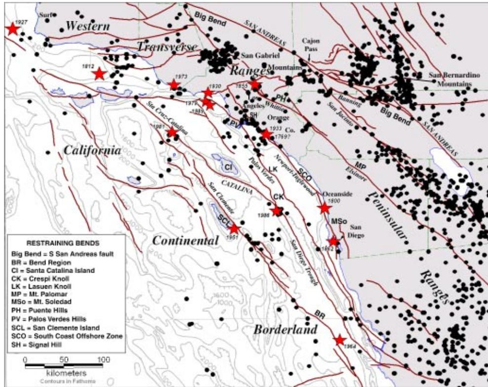
**Figure 1.** Map showing major faults and recent seismicity (magnitude  $\geq 4$ ) of the southern California coastal and offshore region. Epicenters from Southern California Seismograph Network (1932–1998) are shown as small circles; significant offshore historical events are shown as stars. Prominent restraining bends along the major right-slip faults of the region are also identified.
