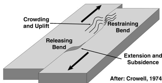
**Figure 2.** Material crowded into a restraining bend along a strike-slip fault results in convergence, folding and reverse faulting that creates a local uplift. In contrast, extension and subsidence occurs at a releasing bend.
