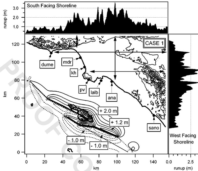
**Figure 5.** Map showing initial wave height for the full seven-segment Catalina Fault model with graphs of runup along the south-facing and west-facing shorelines. Wave gauge locations are plotted and parameters are listed in Table 3.
